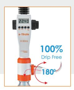
By turning the discharge tube at  $180^{\circ}$  all liquid flows back into the bottle. No more accidental discharge.
