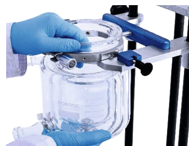
Easy hose clamping and vessel change
