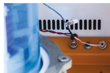
Quick assembly and disassembly using Aviation plugs
