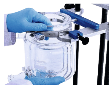
Easy hose clamping and vessel change
