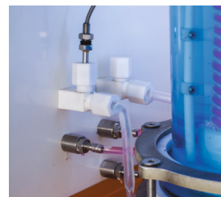
Live monitoring of input and output chiller temperature
