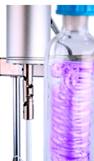
Non-sparking motor drive
