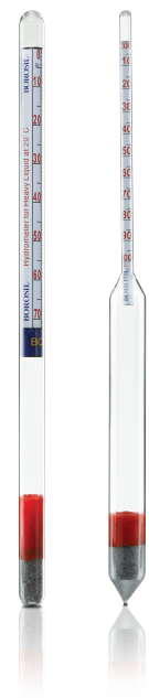
Hold the hydrometer by the top & put into test jar
