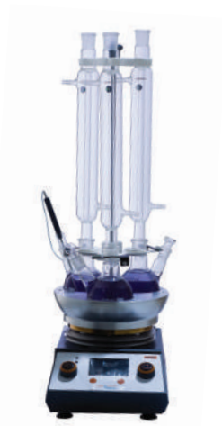
Block Reactor System
