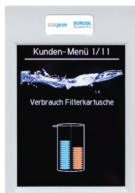
Residual cartridge volume display
